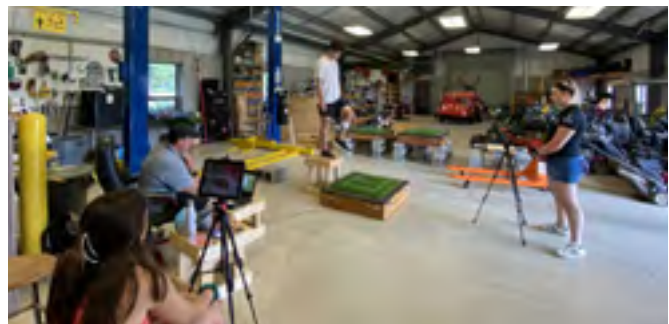
Figure 1. Ground-Reaction Platforms Pictured With the Force Plate and Mobile Motion-Capture System.
